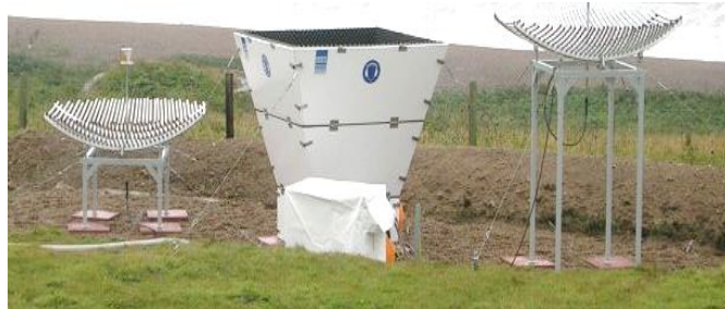
Fig. 1. METEK RAS system based on the PCS.2000 sodar
